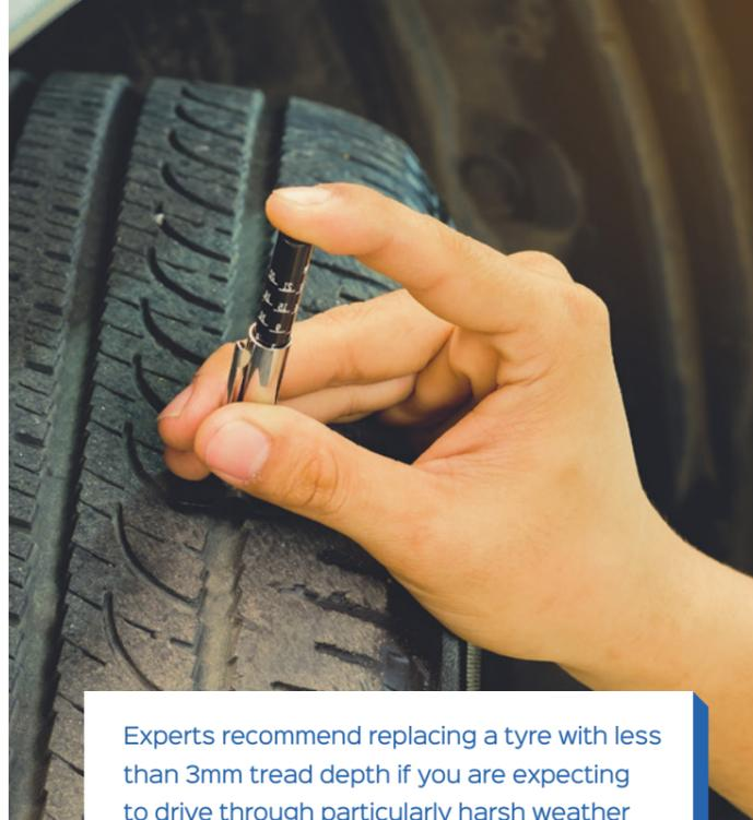
Experts recommend replacing a tyre with less than 3mm tread depth if you are expecting to drive through particularly harsh weather conditions on your road trip.
